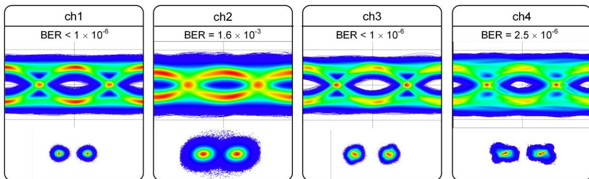
**Fig. 3** Optical eye and constellation diagrams with bit error ratios (BER) of the data experiments (BPSK) at data rates of 10 Gbit/s. All four channels have a BER below the FEC limit of  $2 \times 10^{-3}$ .
