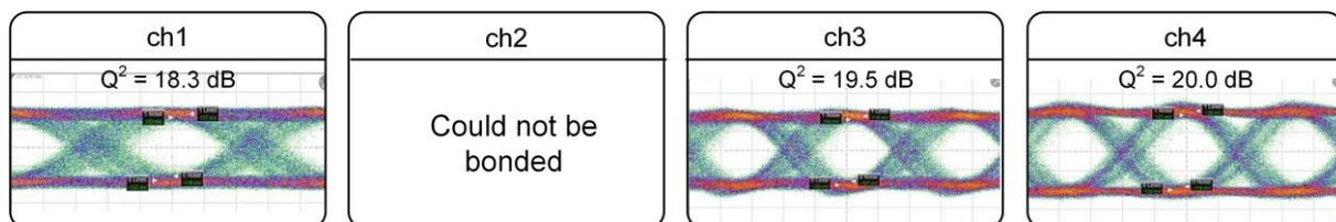
**Fig. 6** Optical eye diagrams with quality factor ( $Q^2$ ) of the data experiments (NRZ, rectangular) at data rates of 28 Gbit/s. Channel 2 could not be bonded (see **Fig. 4**), so no data experiment was carried out. Channel 2,3,4 show open eye diagrams.
