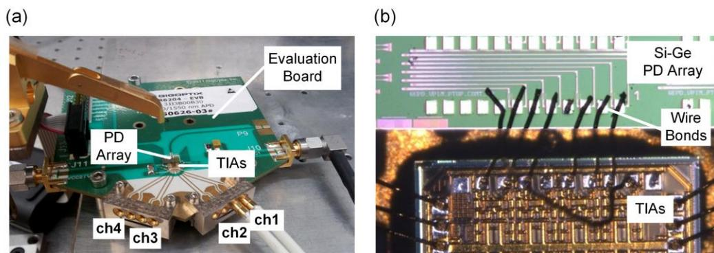
**Fig. 4** Receiver (a) Evaluation board with Si-Ge photodiode array and PCB containing electronics. (b) Photodiodes wirebonded to the PCB. Channel 2 could not be bonded, since the arrangement of the anode and cathode contact pads on the optical and the electronic chip did not perfectly match.
