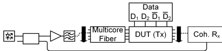
**Fig. 2** Experimental setup for data modulation experiments. Laser light at different wavelengths ( $\Delta\lambda \approx 1$  nm at  $\lambda \approx 1550$  nm) was amplified and coupled via a multicore fiber to the transmitter (Tx). Four electrical data streams were fed to the Tx by two independent DACs. The modulated light of the channel under test was received by a coherent receiver. The laser source was also used as local oscillator in the receiver.
