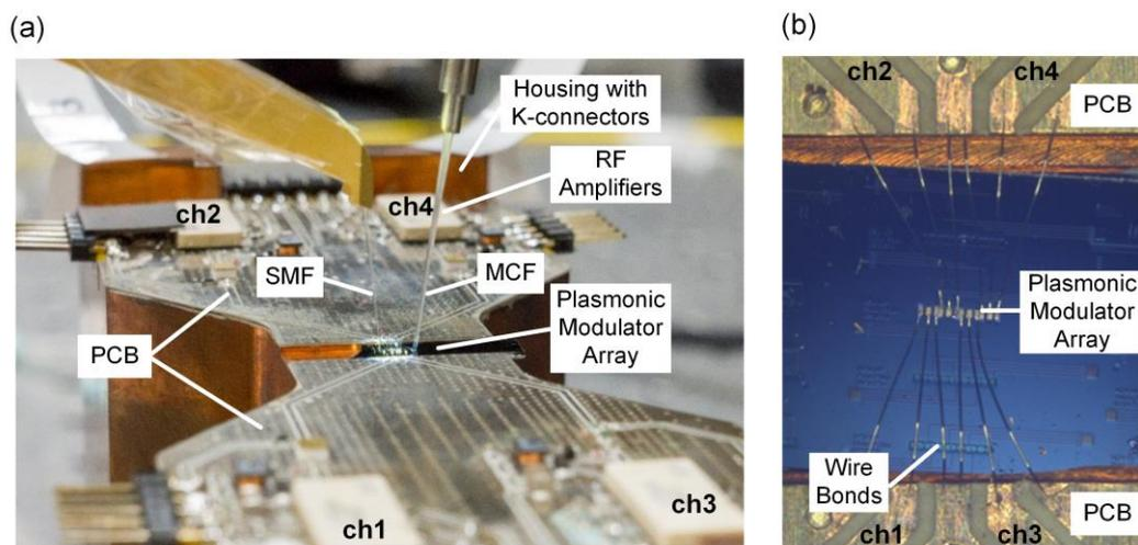
**Fig. 1** Transmitter. (a) Customized package with plasmonic modulator array and PCB containing driving electronics. (b) Plasmonic modulators wirebonded to the PCB.
