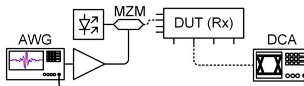
**Fig. 5** Experimental setup for data modulation experiments. Laser light at 1550 nm was coupled to a commercial Mach-Zehnder modulator (MZM). Electrical data streams were generated by an arbitrary waveform generator (AWG) and amplified, before being sent to the MZM. The modulated light was sent to the channel under test of the receiver (Rx). The received signal was measured with a digital communication analyser (DCA).
